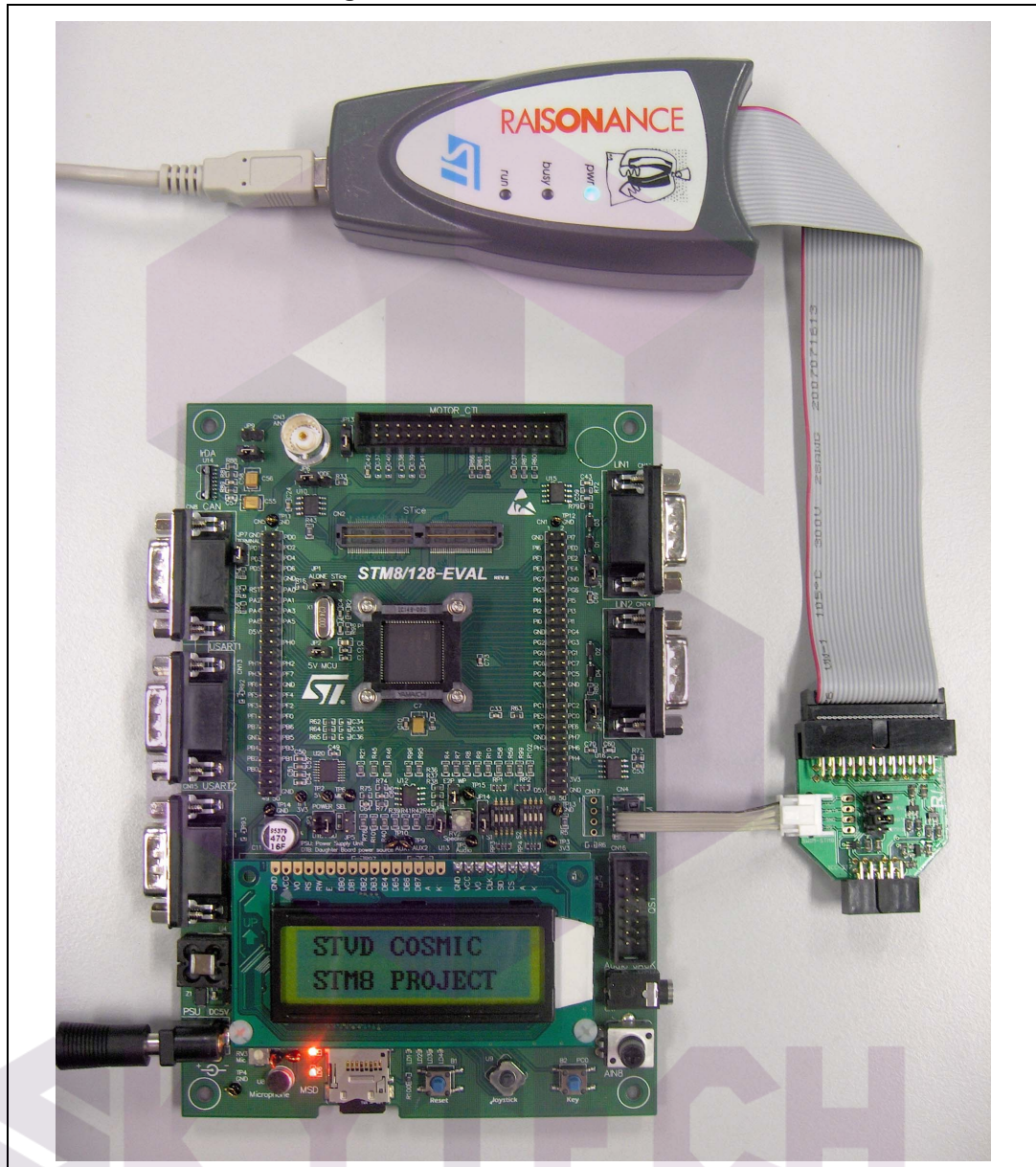
Figure 26. STM8 evaluation board
